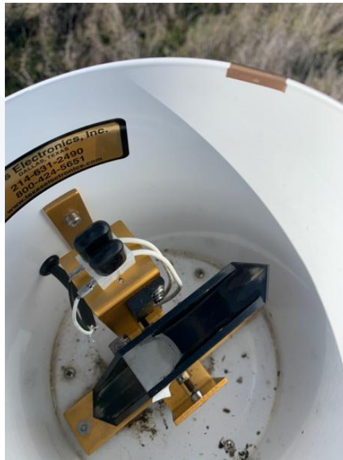
Inside of rain gauge showing tipping bucket mechanism
